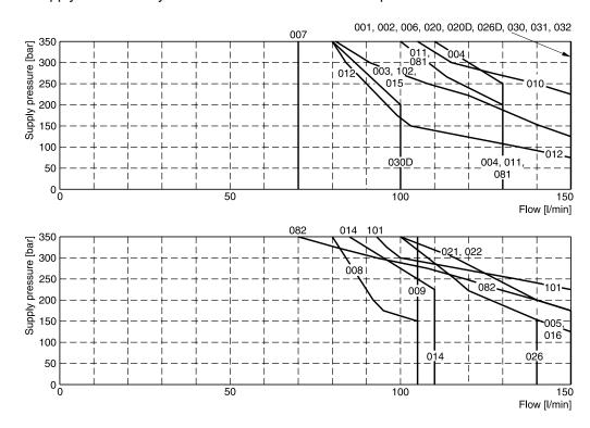
Measured with HLP46 at 50 °C, 90 %  $U_{\tiny nom}$  and warm solenoids.
